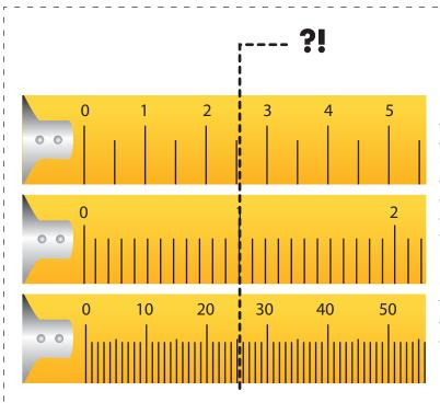
Length can be measured in three common units – millimetres, centimetres and metres. Most trades use millimetres, but domestic tape measures use centimetres. Several different systems are used to mark millimetres and centimetres on standard measuring tapes.
